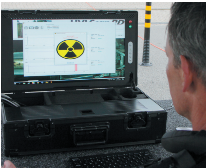
UVIScan® Rapid Deployment workstation displaying UVIScan® Gamma alarm.
